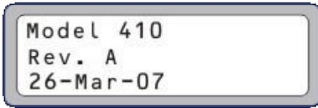
To display the revision page, press the Right arrow key when Units is the highlighted parameter.
