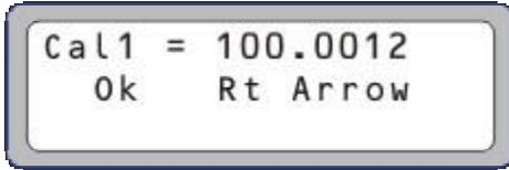
The current calibration point and suggested calibration value (0 ohms for cal point #0 or 300 ohms for cal point #1) are displayed. The actual calibration resistance value should be within 1 or 2 percent of the suggested value and known to within 0.0010% (10 ppm).
